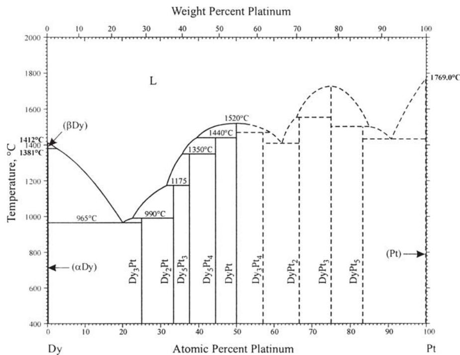
**Fig. 1** Dy-Pt phase diagram
